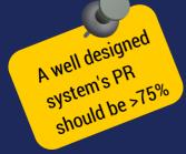
Typically, PR should be measured over an entire one year period. \*Commercially available PV module's efficiency is around 15-16%
